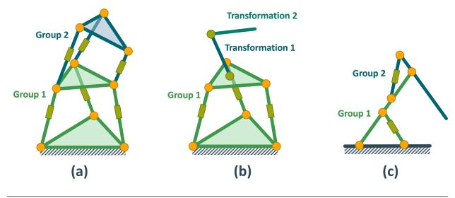
The excavator has two actuated states and two virtual states. These are the lengths of hydraulic cylinders  $a_1$ ,  $a_2$  and the arm angles  $q_1$ ,  $q_2$ . Since each cylinder length  $a_i$  controls one arm angle  $q_i$ , the excavator can be divided into two groups. These are visualized by the green and blue parts respectively.
