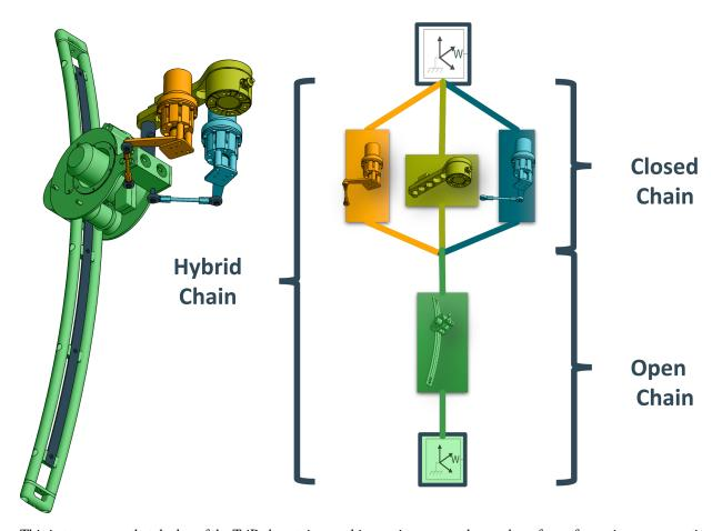
This in turn means that the leg of the TriPed contains one kinematic group and a number of transformations representing the open chain.
