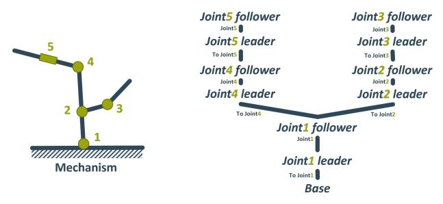
Here the cursive graph nodes are coordinate frames while the edges are the transformations between them. Since TriP only models transformations and not coordinate frames in TriP the name of a coordinate frame is synonymous with the name of the transformation leading to it. This leads to the following simplified transformation tree:
