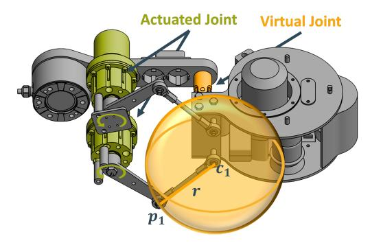
The mapping between these joints can be computed by solving a geometric closing equation. As pictured above, the tip  $x_i$  the output lever connected to the actuated joints i always intersects the sphere at position  $c_i$  where i is either 1 or 2.
