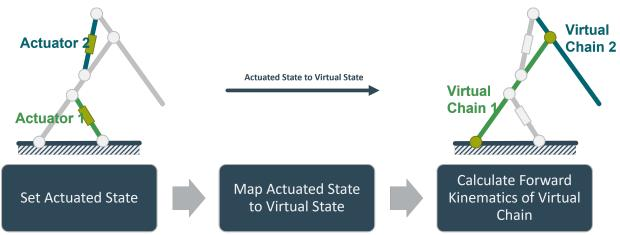
The forward kinematics of the virtual\_chain are in this case calculated by multippling the transformation matrices of the virtual\_chain together. This results in a 4x4 transformation matrix describing the state of the end effector.
