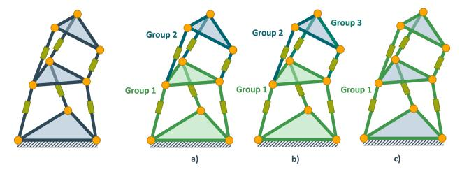
Grouping a) and c) are valid groups, with a) being more performant. However the Grouping in b) is not valid. The reason is that the state of the top platform depends on the state of all three green prismatic joints.
