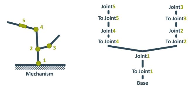
In this tree the edge and the node it leads to refer to the transformation. TriP builds this simplified transformation tree by specifying the parent of each transformation. The parent is in this case the transformation that preceded the current transformation. For the example transformation tree this would look like this:
