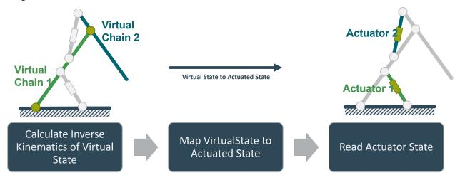
First, the system tries to find a virtual state which results in the end effector being as close as possible to the target. This is done using a casadis NLP solver using auto-generated jacobian and hessian matrices.
