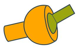
actuated\_state = {spherical\_1 :  $\theta_x$ , spherical\_2 :  $\theta_y$ , spherical\_3 :  $\theta_z$ } virtual\_state = {spherical: { rx :  $\theta_x$ , ry :  $\theta_y$ , rz :  $\theta_z$ }}
