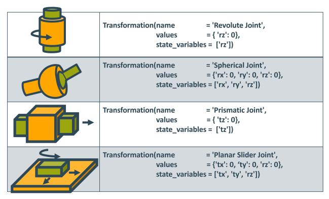
Note that while all non specified parameters are assumed to be zero, the value of each *state\_variable* still has to be supplied.
