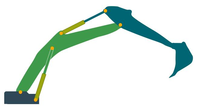
In this example, multiple coordinate systems have more than one parent since the transformations form a loop.
